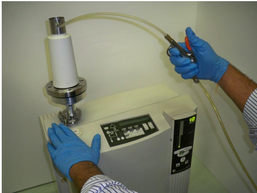
Helium Leak Check of Ceramic Metal Vacuum Feed-Thru
